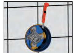
Trim the protruding part of the box, turn off the water and disassemble the flushing device.
